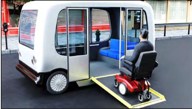
*The ADA Guidelines require ramps to have a clear width of at least 30 inches, edge guards at least 2 inches high and visual contrast striping along the perimeter of the ramp.*
