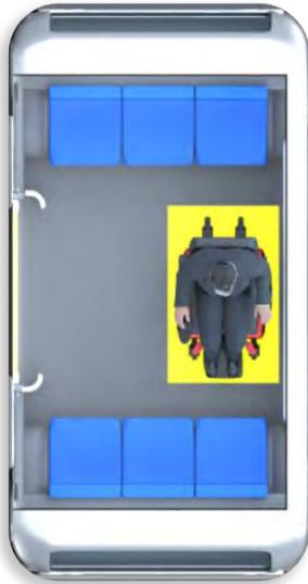
These provisions specify sufficient clearances that allow passengers using wheelchairs and power chairs to proceed from vehicle entry to designated wheelchair spaces, position for securement within the space, and exit the vehicle. Wheelchair turning space is recommended, though not required, to provide greater maneuverability and usability.
