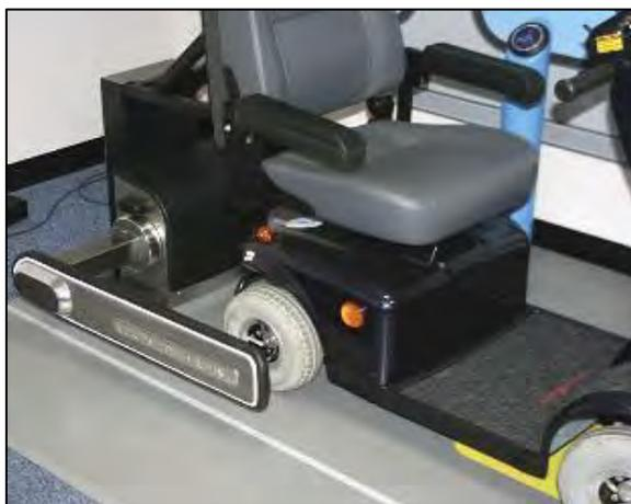
*Q'Straint's QUANTUM securement system*
