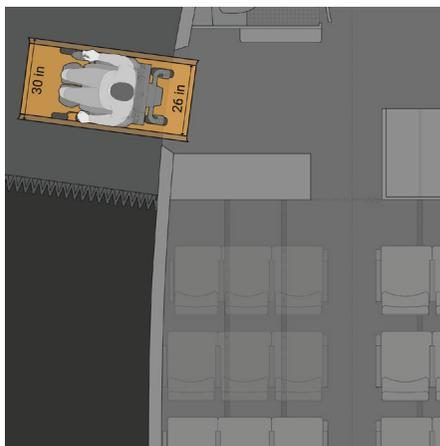
FIGURE 4-9 Forward boarding door clearances, Boeing 737.
