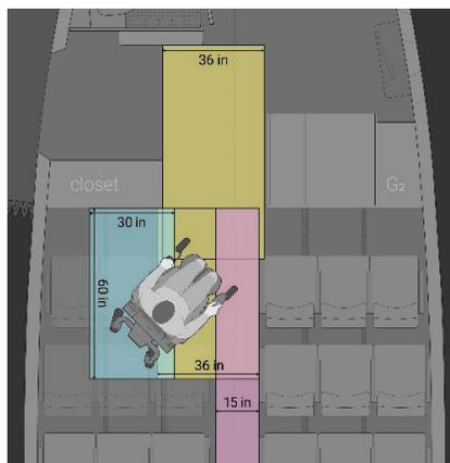
FIGURE 4-11 Space for a wheelchair maneuvering laterally between the aisle and securement area, Boeing 737.
