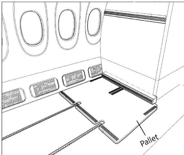
FIGURE 2-9 Aluminum pallet for distributing load across airplane floor structure. SOURCE: European Patent Application.<sup>17</sup>
