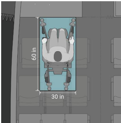
FIGURE 4-6 Space required for the securement area.
