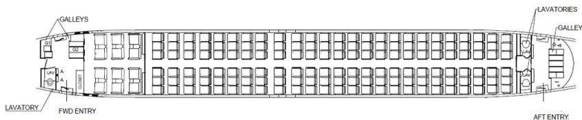
FIGURE 4-8 Boeing 737 interior layout with first class seating.
