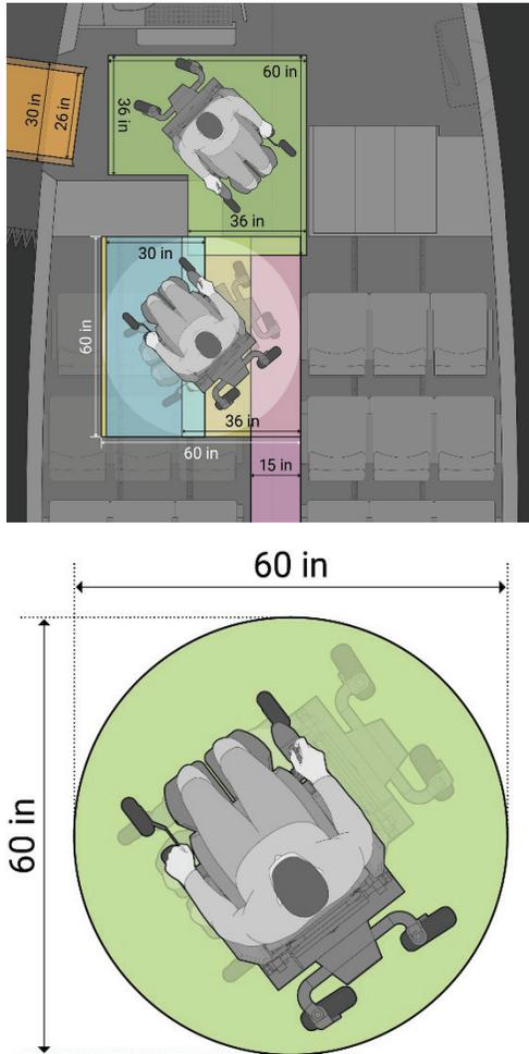
**FIGURE 4-7** Minimum space required in the securement area and adjacent aisle to turn the wheelchair around to a front-facing securement position after entering facing forward.
