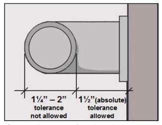
Construction or manufacturing tolerances are permitted for the required clearance at grab bars since this is an absolute dimension (1½ inch), but they are not permitted for the grab bar diameter because a range is specified (1¼ to 2").
