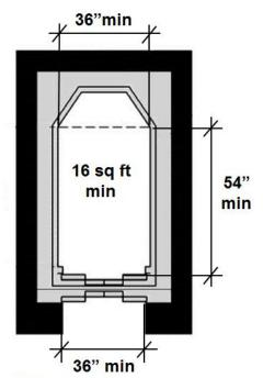
(32" min if door power operated and door/hoistway depth is 24" max )
