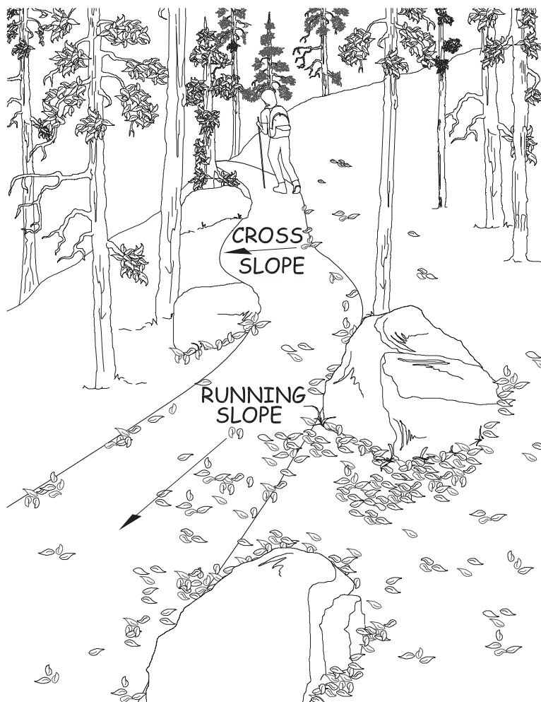
Figure 8—The running slope is measured along a trail’s length; the cross slope is measured across its width.
