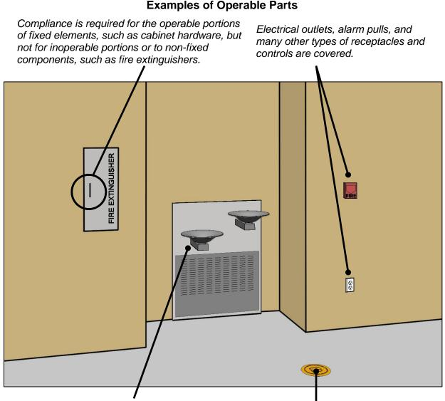
Provisions for drinking fountains and other elements covered by the standards also apply the criteria for operable parts. Exempt: floor receptacles and operable parts used only by service or maintenance personnel.
