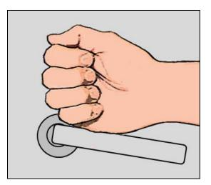
Operability with a closed fist is a reliable test of usability, but is not required by the standards.
