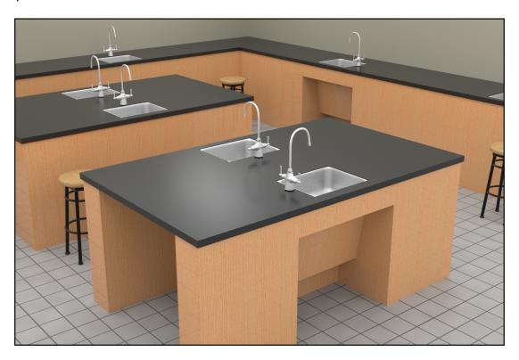
At least 5% of sinks, but no less than one sink of each type, must comply in each accessible room or space, such as classroom labs (§212.3). At least 5% of work surfaces must also comply (§226.1).
