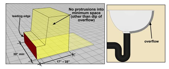
Beyond a depth of 8" measured from the leading edge, the 27" minimum high knee clearance can reduce 18" to a height of 9" minimum (toe space) over a 3" span (6:1 slope). When the knee and toe is deeper than 17", the additional depth must provide full knee clearance at least 27" high.
