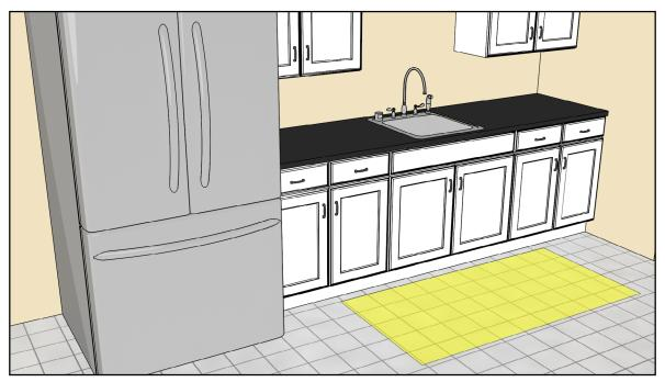
A parallel approach is permitted at kitchen sinks (i.e., sinks used for food preparation) located in breakrooms, kitchenettes, and similar spaces that do not have either a cooktop or conventional range (§606.2, Ex. 1).
