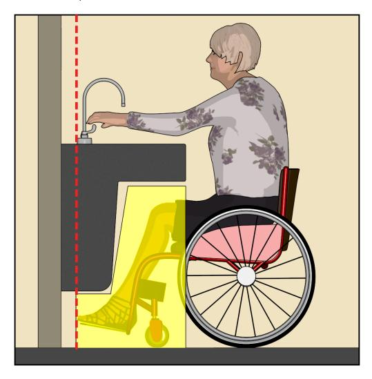
To avoid issues with garbage disposals protruding into knee and toe space, use a sink with a drain located at the rear of the bowl instead of the center. At sinks with two bowls, knee and toe space is required beneath only one bowl (§606.2, Ex. 7).
