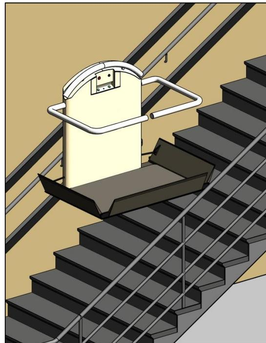
*Inclined platform lifts can have a folding platform and are typically located at stairways. They must be installed so they do not encroach on required means of egress. Passenger retaining arms are permitted as an alternative to a platform enclosure under the ASME A18.1 Standard.*
