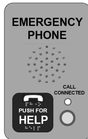
*The ASME A17.1 code addresses features of required two-way emergency communication devices, including controls and visual indicators. The ABA Standards apply requirements for operable parts and tactile characters and symbols.*
