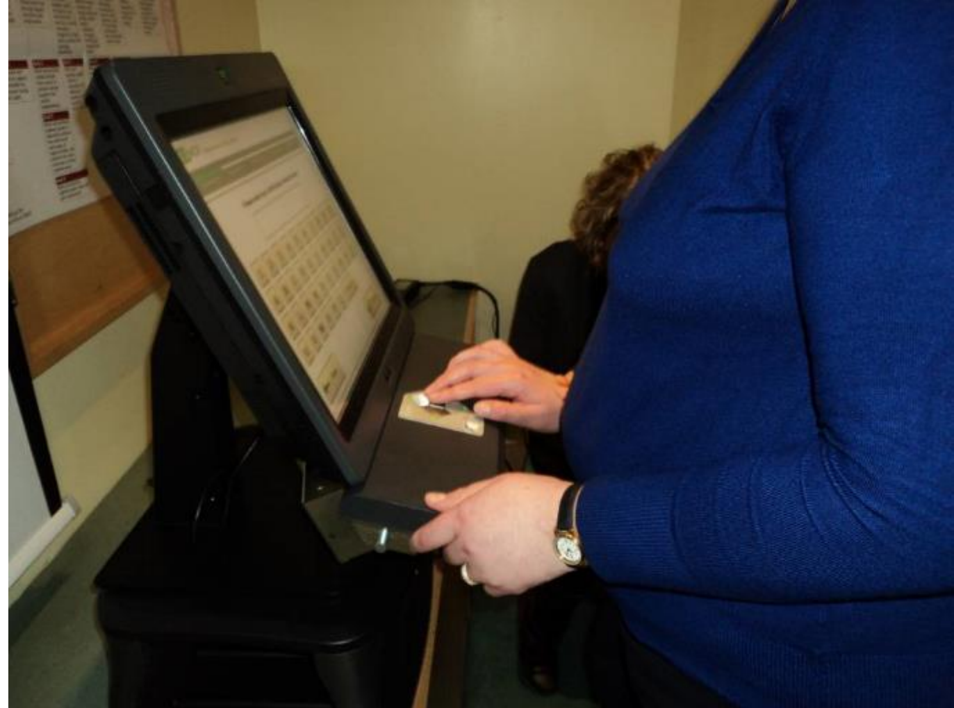
Photo of a person using a prototype uNav on a shelf below a 15" touchscreen displaying an onscreen keyboard
