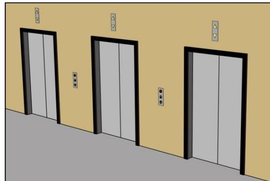
*When an alteration is made to an existing car, it also must be made to all other cars that respond to the same hall call.*
