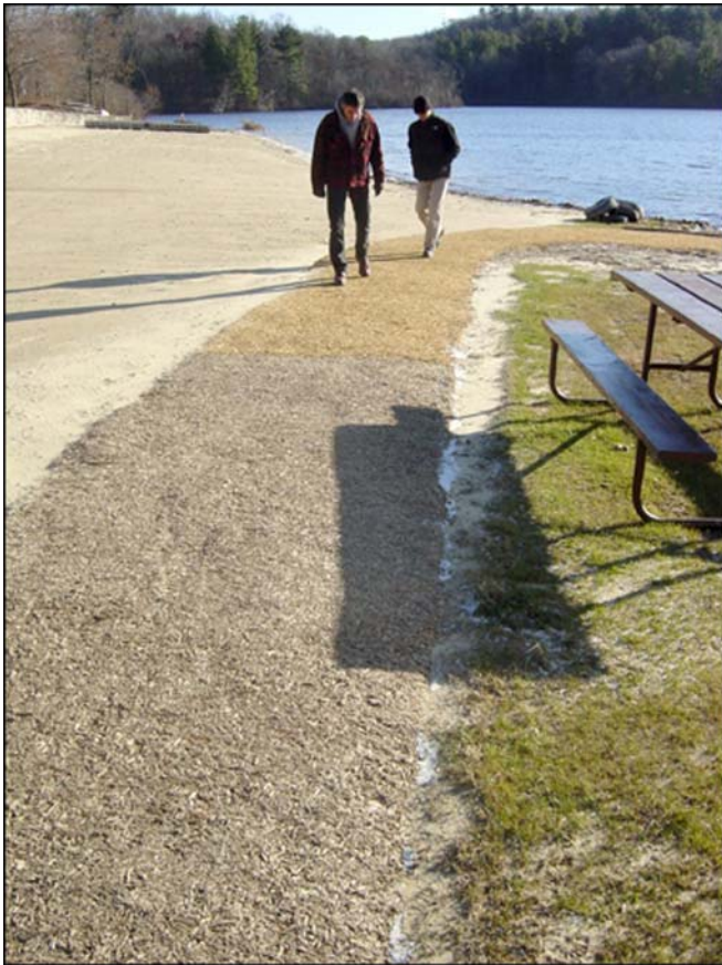
Figure 7—Beach path after 2 months of weathering. Junction of Soil-Sement and Vitri-Turf surfaces is just above the shadow cast by the picnic bench.
