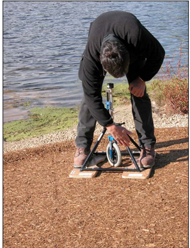
Figure 14—Rotational penetrometer used to measure accessibility.
