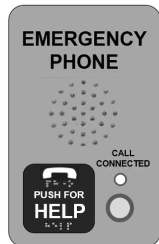
*The ASME A17.1 code addresses features of required two-way emergency communication devices, including controls and visual indicators. The ADA Standards apply requirements for operable parts and tactile characters and symbols.*
