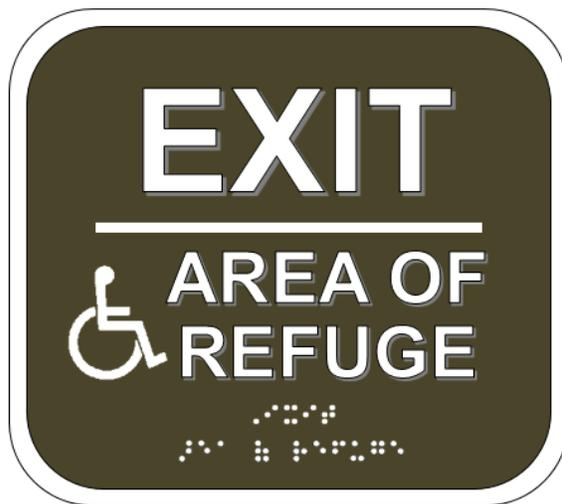
*Area of refuge signs can be incorporated into required exit signs. Requirements for tactile signs address raised characters, braille, finish and contrast, separation from raised borders, and location (i.e., 48” – 60” AFF measured to the baseline of raised characters), and other features.*
